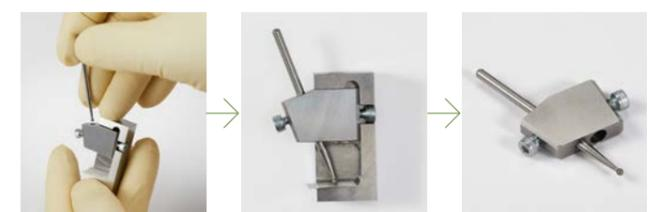
**Setting the bit** Place a sheet of thin paper at the bottom of the height adjustment jig where the bit touches it. Screw the bit and remove the head from the jig.
