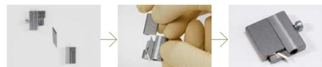
**Attaching a cutter** Set the cutter to the head. Put a cover for protecting the cutter from falling off.
