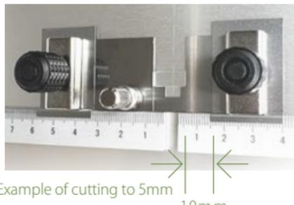
Use magnetic substrate guides to hold the substrate from both ends.
