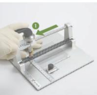
Fine tune the height by cutting an actual sample to find the best position of the
